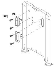
• Attach two locks (#5) to the outside of each pedestal using bolt (#29) .
